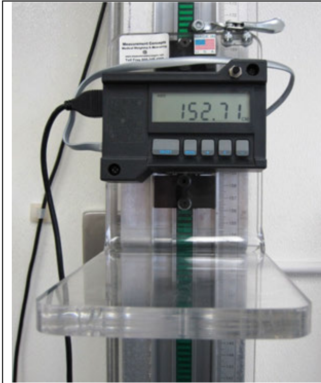
Exhibit 2-7. Stadiometer headpiece and digital measurement device
